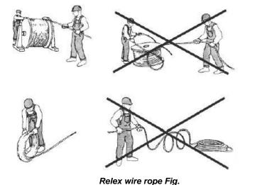
During the installation process knot is due to incorrect Matsunawa methods or did not pay attention to some of the spinning rope to stay on top in the production process. If this is the case to get the rope (pictured), the rope should begin around and restored to its original shape from its end.
