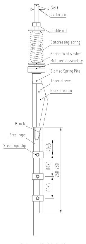
Wedge rope fixed device Fig.
