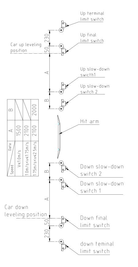
Terminal switch layout Fig. (Refer to electrical manual)
