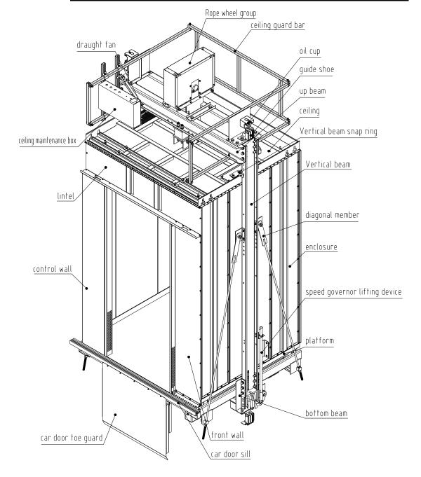
Car frame system schematic fig
