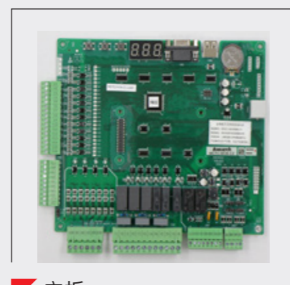
主板 Main Board 确认产品型号、是否带协议，程序版本、是否有非标。 Confirm the model, if it's with protocol. Confirm the procedure version, if it's non-standard.
