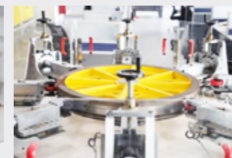
扶梯滚轮检测 Escalator Roller Test
