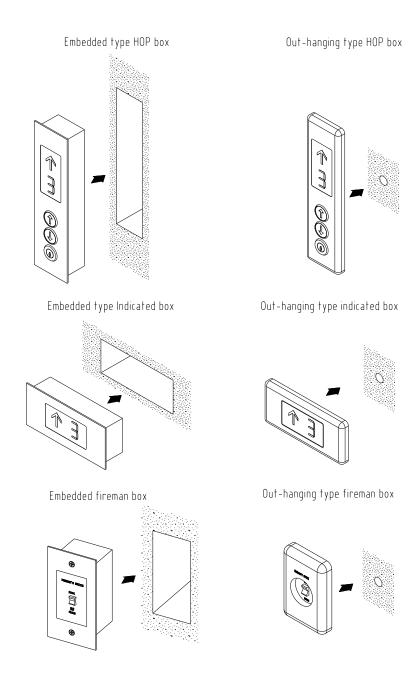
Installation of HOP box, floor indicated box, fireman box Fig
