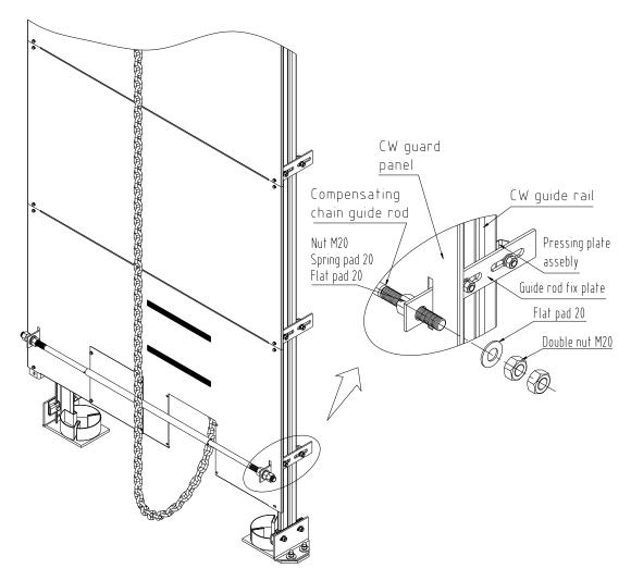
Installation of compensating chain guide rod Fig.
