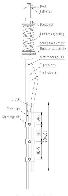
Wedge rope fixed device Fig.
