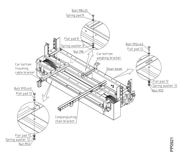
nstallation of travelling cable hanging bracket, compensating chain hanging bracket Fig
