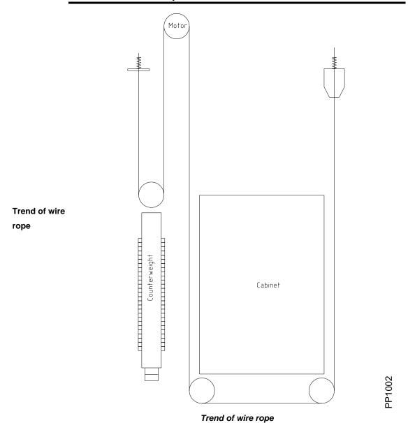
Installation of wire rope
