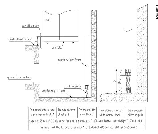
Calculations of counterweight supporting bracket's height fig (e.g. lower part of counterweight with scaffold construction)
