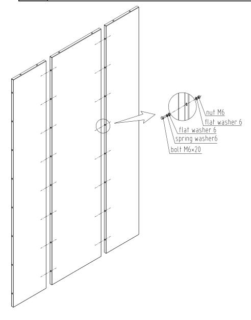
Installation of side wall and rear wall fig
