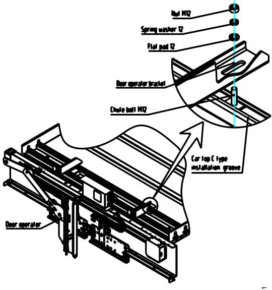
Installation of CO door operator Fig.
