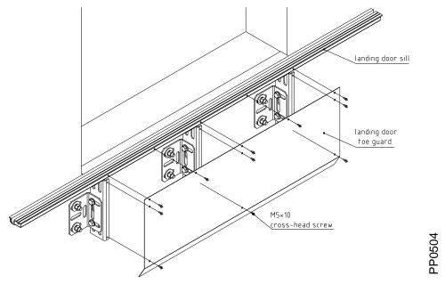
Installation of sill toe guard fig
