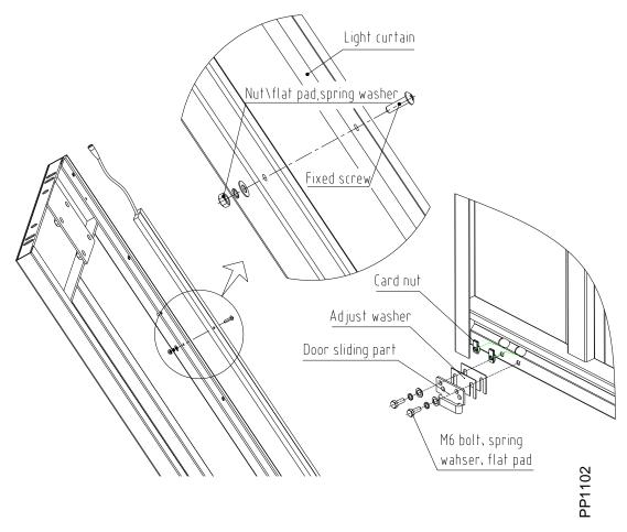
Installation of car door and light curtain Fig.
