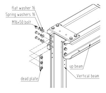
Installation of the up beam , lower frame and stile fig
