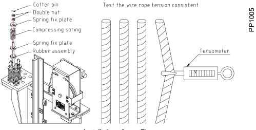
Installation of rope Fig.
