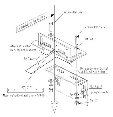
Car guide rail bracket fixation installation fig
