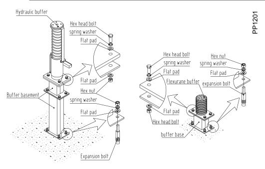
Installation of buffer Fig.
