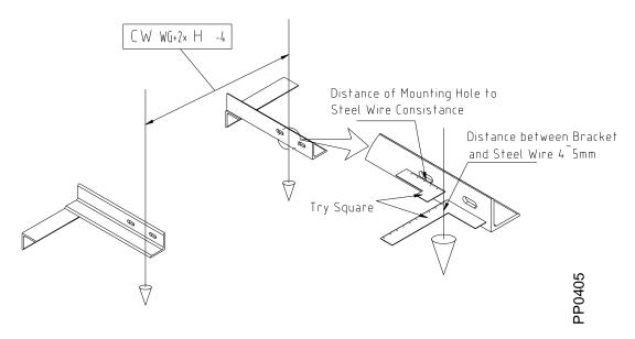
counterweight guide rail bracket fixation fig
