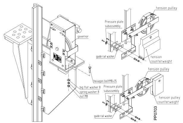
Installation of governor and tension pully fig
