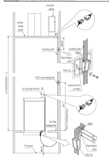
Installation of travelling cable Fig.
