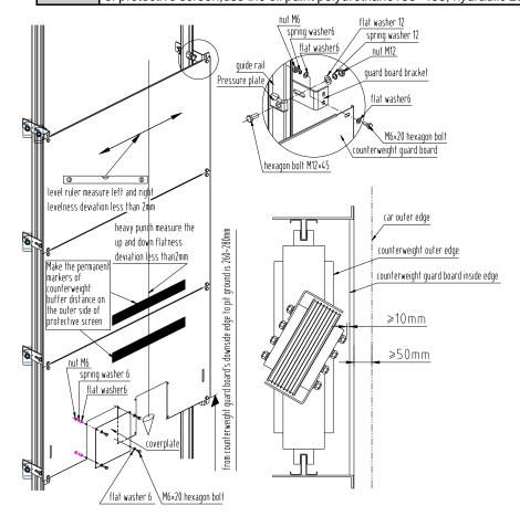
Installation of counterweight protective screen fig
