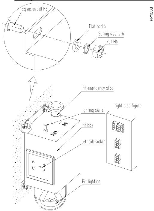
Installation of pit inspection box fig.
