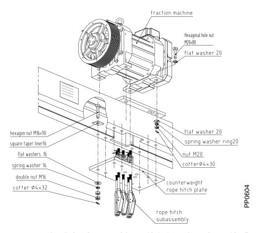
Installation of counterweight rope hitch plate and traction machine fig
