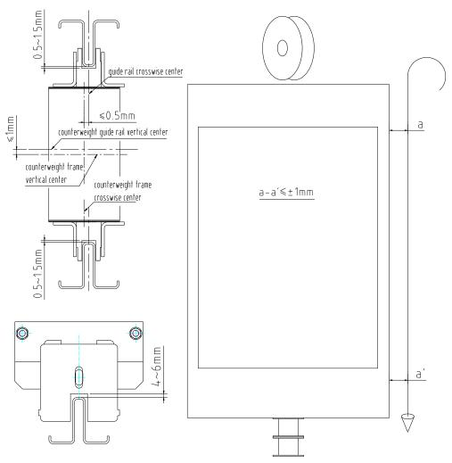
Adjustment of counterweight frame, guide shoe and oil cup fig
