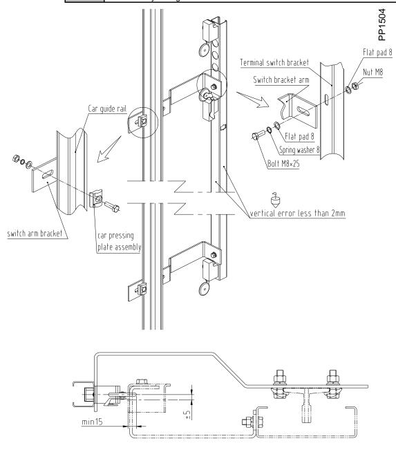
Installation of up terminal switch Fig.
