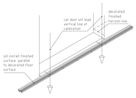
Center opening sill marking line fig
