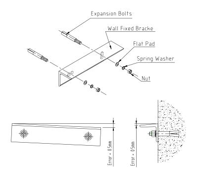
Wall Fixed Bracket Error Adjustment Fig
