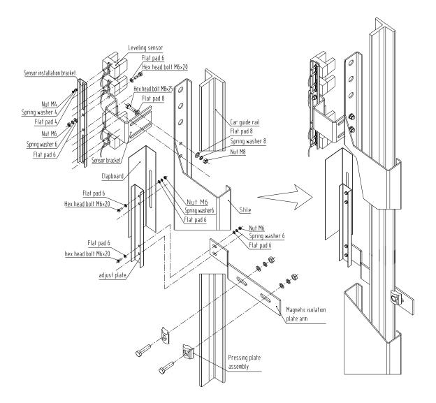
Installation of leveling sensor Fig.
