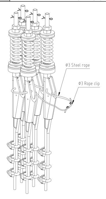
Installation of rope anti-reverse Fig.
