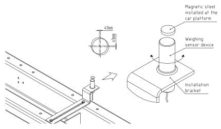
Installation of weighing switch Fig.
