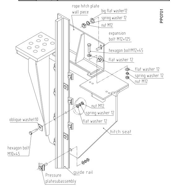
Installation of speed governor hitch beam fig
