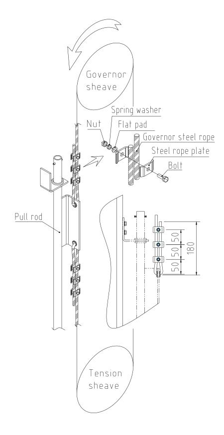
Connection of speed governor rope and pull rod Fig.
