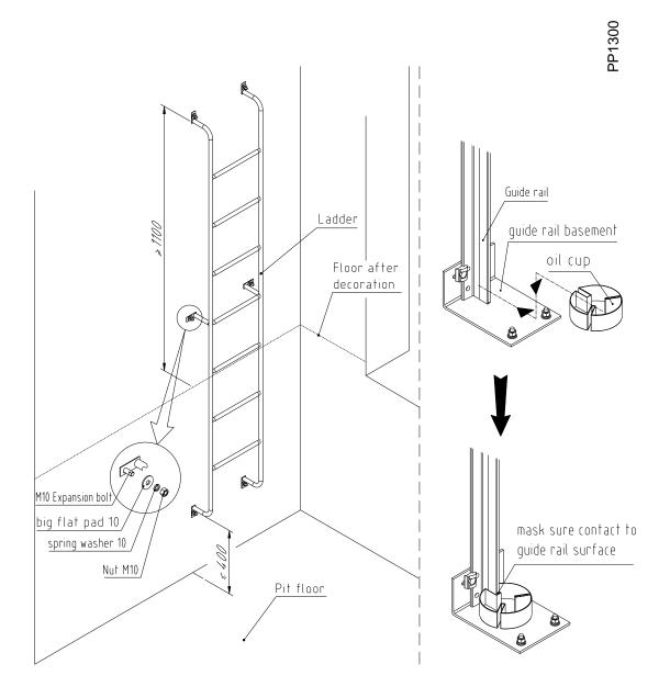
Installation of pit ladder and oil collected box Fig.
