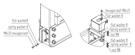
Installation of counterweight guide shoe and oil cup fig
