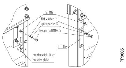
Fixation of counterweight frame side hood and counterweight filler pressure plate fig 8.4 Installation of counterweight protective screen.
