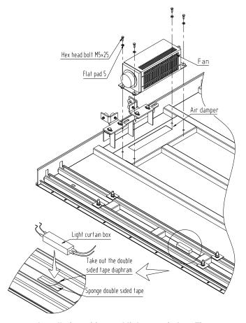
Installation of fan and light curtain box Fig.
