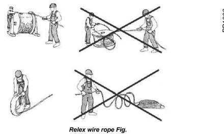
During the installation process knot is due to incorrect Matsunawa methods or did not pay attention to some of the spinning rope to stay on top in the production process. If this is the case to get the rope (pictured), the rope should begin around and restored to its original shape from its end.
