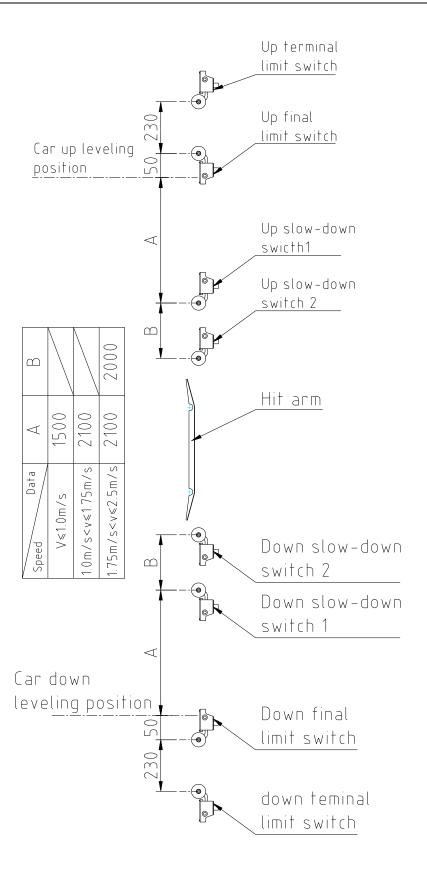
Terminal switch layout Fig. (Refer to electrical manual)
