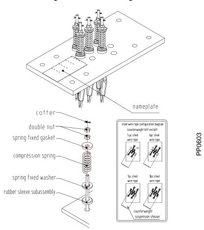
Pre-installation of rope head component fig
