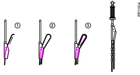
Installation of rope socket and wire rope Fig.
