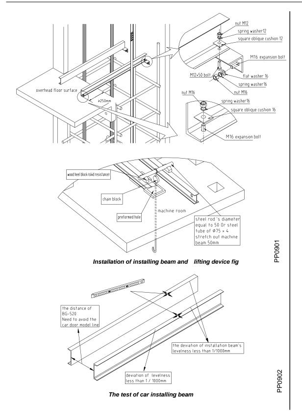
9.2 Installation of the up beam, lower beam and stile
