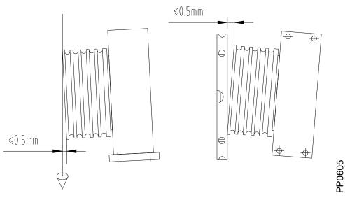
Adjustment of traction machine fig
