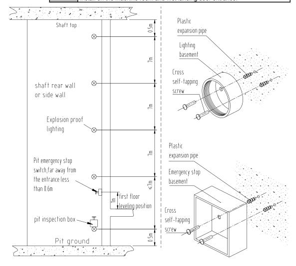
Installation of shaft lighting and emergnecy switch Fig.
