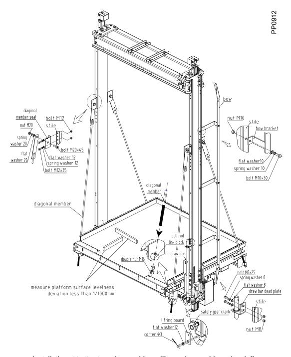
Installation of inclined rod assembly, pulling rod assembly and arch fig
