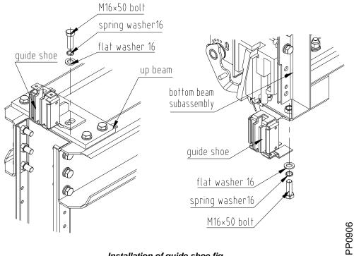
Installation of guide shoe fig
