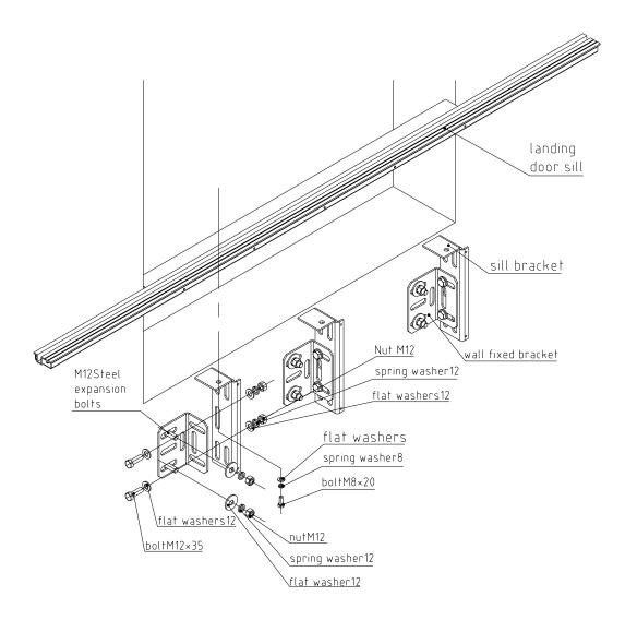
Installation of sill subassembly fig
