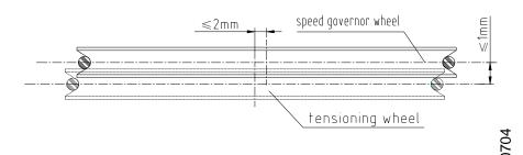
Adjustment of speed governor and tensioning wheel fig
